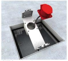
2 | CEE-Connection socket Detach CEE socket from box and device carrier by unscrewing four screws. Insert rubber seal. Insert connecting cable into container and clamp to CEE box. Reassemble device carrier completely.
